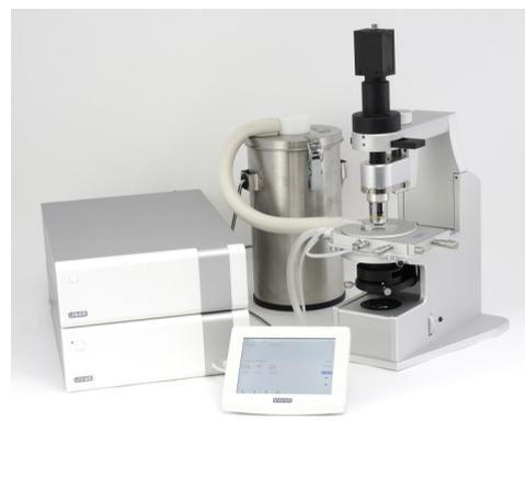
THMS600 stage with T95 LinkPad and LNP95 cooling
